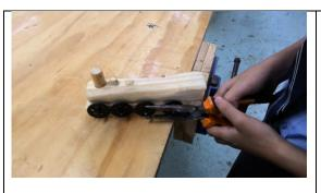
Here I am using pliers to cut the plastic axels to size, because it allowed for precise and safe cutting of the axels and rubber stoppers.
