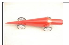
This dragster has a conic shape and rubber-coated wheels, which makes it very aerodynamic, however it is not made of wood, which is the permitted material. Additionally, it has a very simple design which is not aesthetically pleasing. The car also has an extension on the back to fit the CO2 canister instead of a hole drilled into the body of it.
