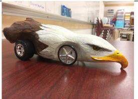
The dragster in this image looks like an eagle, which is very visually pleasing and aesthetic. However, the beak touches the ground, providing friction and less aerodynamics. The rear wheels being wrapped in more rubber than the front wheels is an interesting design choice that may help improve the dragster's stability when raced.
